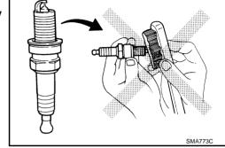
Checking and adjusting plug gap is not required between change intervals.
