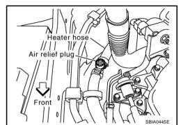
Fill radiator with water until water spills from the air relief hole, then close air relief plug. Fill radiator and reservoir tank with water and reinstall radiator cap.
